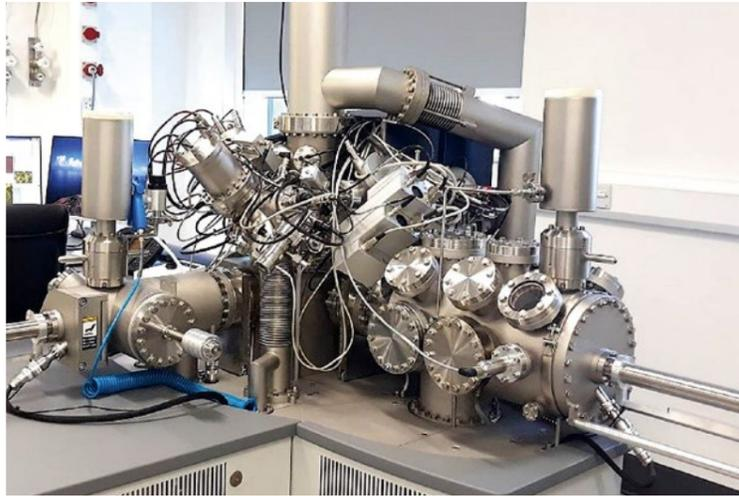
Time-of-Flight Secondary Ion Mass Spectrometry (ToF-SIMS) equipment
