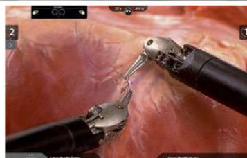
holders with a complex Bowden pulley mechanism are used. This construction, which is necessary for the robot to be able to position the instruments more precisely in the body, comes with a drawback, Knobloch finds: 'Cleaning and disinfecting is much more complicated
