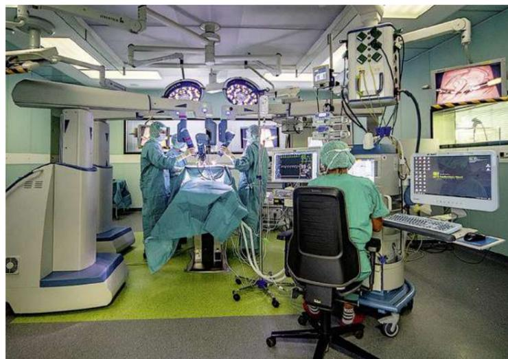
cedures in general and visceral surgery was introduced in Wesel at the beginning of August. It provides the surgeon, who sits next to the patient in a comfortable position at an open console during the operation, with pin sharp, high resolution images enlarged up to six times. The camera is controlled with the surgeon's eye movements, the instruments inside the patient's abdomen are controlled via the hands. An
