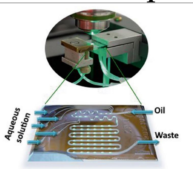
Figure 1: *Lab-on-a-Chip* SERS platform developed at Leibniz-IPHT Jena. Above: Photo of the lab setup. Below: Illustration of the microfluidics chips with aqueous droplets in the oil flow.
