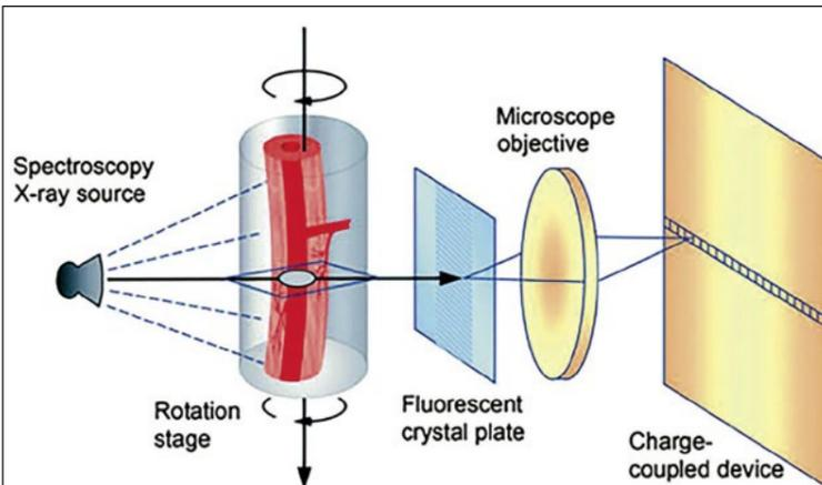
Schematic diagram of the microcomputed tomography device (micro CT). CCD = Charge-coupled device.
