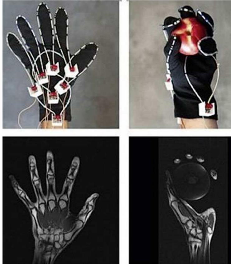
A flexible MRI detector array in the form of a glove. Top: photos of the hand in various poses. Bottom: corresponding MR images obtained using the glove. With multifaceted sensor technology like this, MRI can embrace new flexibility.
