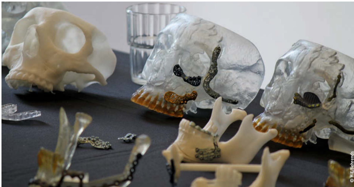
Cranio-maxillofacial plates have been among the first medical implants to benefit from 3D printing technology at scale.
