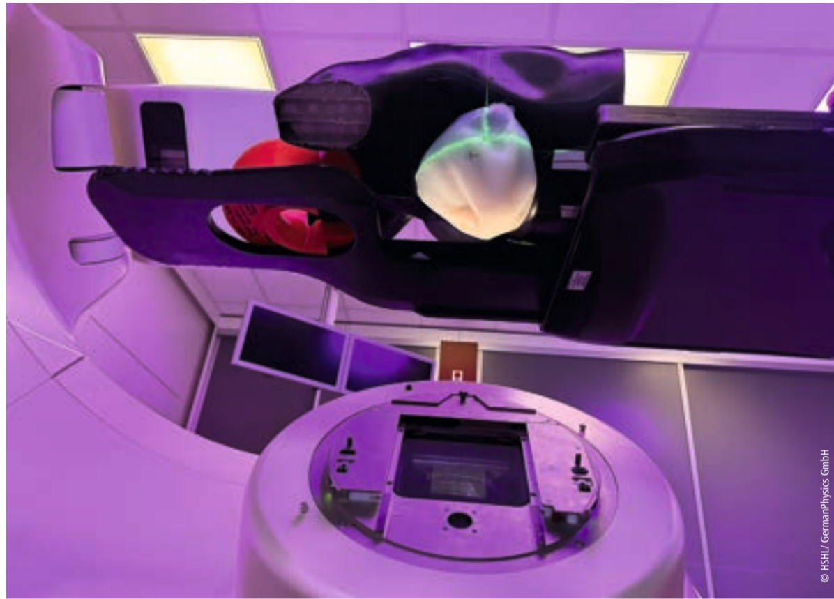
X-Akt Mamma RTX with breast phantom during a radiotherapy session
