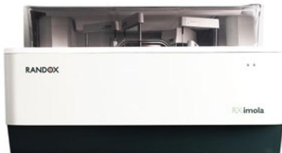
**Sample throughput:** 400 photometric tests per hour, 240 ISE tests per hour
