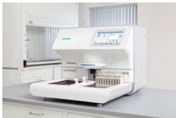
**Highlights:** The CLINITEK Novus Automated Urine Chemistry Analyzer combines proven dry-pad urine chemistry technology with an easy-to-use cassette test format to help ensure standardized testing and maximum productivity in busy laboratories.
