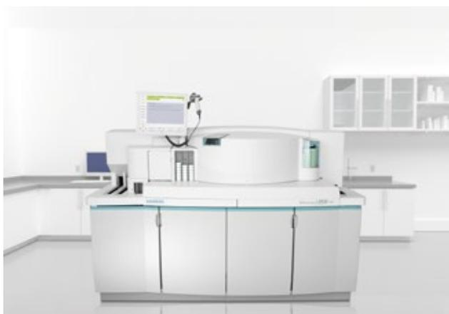
**Sample throughput:** Up to 2000 tests/h (Dimension Vista 1500)
