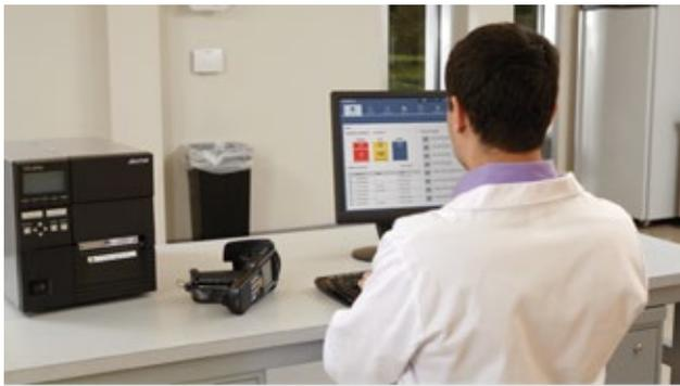
**Highlights:** sLIM is a real-time inventory-management system that employs cloud-based technology and wireless radio frequency identification (RFID) to master laboratory inventory management. Incoming inventory is checked into your laboratory's sLIM website. sLIM automatically detects inventory usage, eliminating manual counting, and recording. Automated order proposals are generated based on your laboratory's usage. sLIM takes the burden out of managing inventory.
