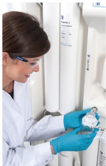
A sanitary sampling valve can provide easy and reliable microbiological testing of analyser feed water produced by the water purification system
