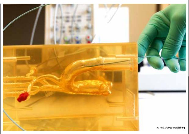
The image shows a catheter phantom. It describes a typical case where a catheter equipped with a millimetre-wave sensor system could be used. The scale becomes particularly clear: the phantom is oriented on the original size. The sensor to be developed needs to fit into the small catheter-top to detect fatty- and calcareous plagues in the arteries.
