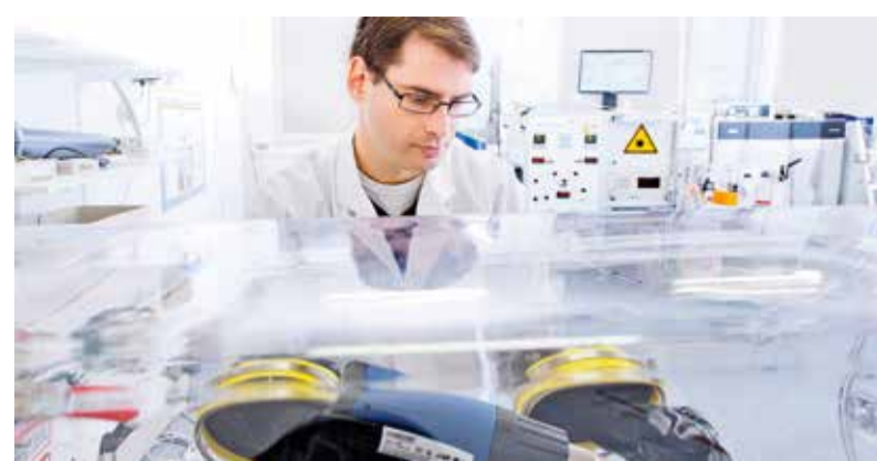
Physicist Leif Schröder preparing a rubidium sample under protection atmosphere for the laser setup to generate hyperpolarised xenon for novel MRI applications.
