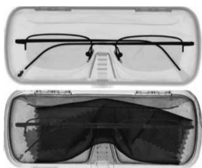
Image of the spectacles case from the new technology (bottom) reveals the cleaning cloth
