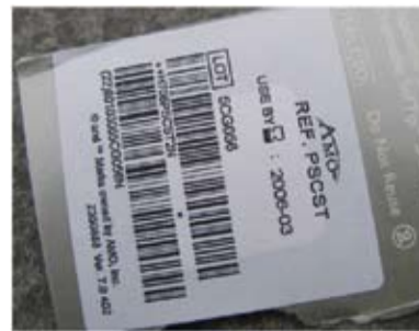
Example 3: Disposable attachment ophthalmology Negative: Content is not indicated on the label, oversized barcodes
